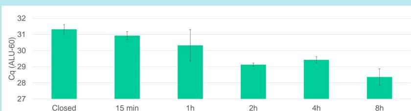
**Fig 2. Contamination control of eppendorf tube used for mastermix preparation.** The tubes were left open to the atmosphere for various amount of time (0, 15 min, 1h, 2h, 4h and 8h), and contamination was measured with TATAA ALU-60 assay.
